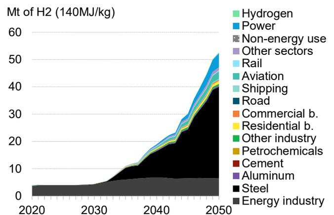
Source: BloombergNEF, IEA. Note: ‘Energy industry’ includes legacy uses (especially as feedstock for ammonia and methanol production or in oil refining) as well as own-use for energy producing industries, such as process heating, lighting, and equipment operations. Commercial b. – Commercial buildings, Residential b. – Residential buildings.
